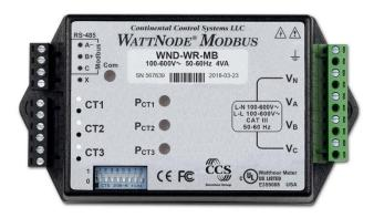
The WattNode® Wide-Range Modbus Meter measures bidirectional energy, power, voltage, current, etc. It communicates using Modbus® RTU over RS-485. The WattNode Wide-Range provides revenue-grade system accuracy when used with the CCS Accu-CT® family of revenue grade (C0.6 or better) current transformers.
